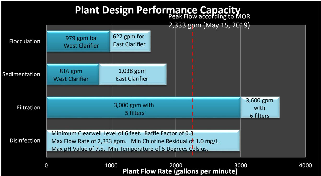
Figure 7: The calculated capacities of each major unit process
