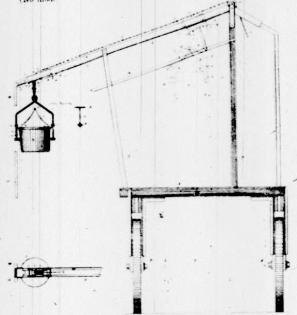
Chim.—1. The combination of a hoisting-bucket having a bail pivotally connected thereto below its center of gravity, a locking device for locking said bucket from turning on its bail, and a tripping-lever pivoted to a suitable support adjacent to the bucket's dumping position adapted to be operated by the bucket to trip said locking device, substantially as described.
