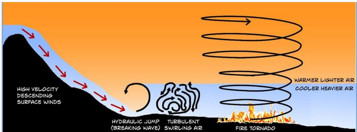
Figure 3- Hydraulic jump illustration
