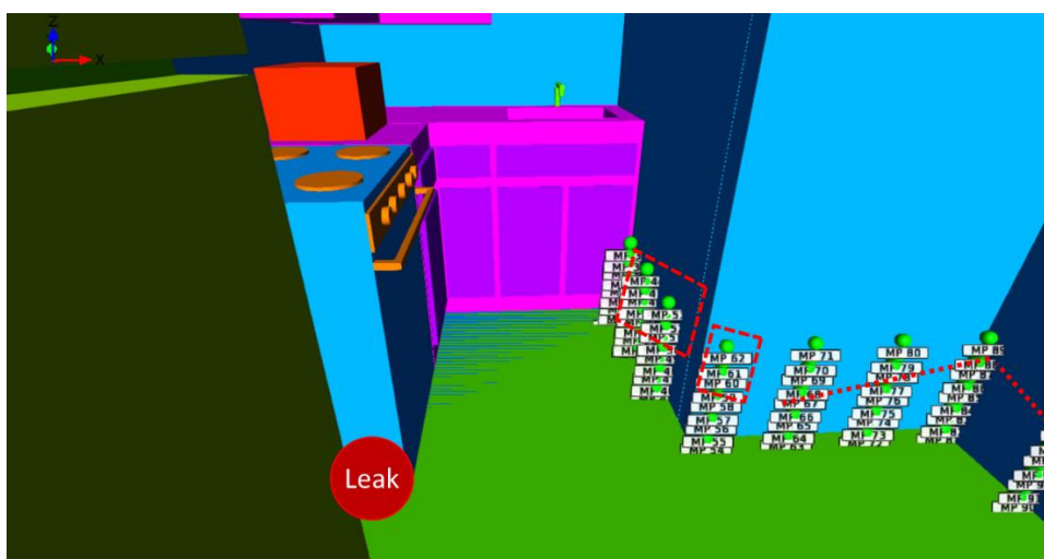
Figure 4.20: Locations which did not activate prior to threshold conditions in the townhouse kitchen - detectors above the horizontal dashed red line and those contained within the boxes.
