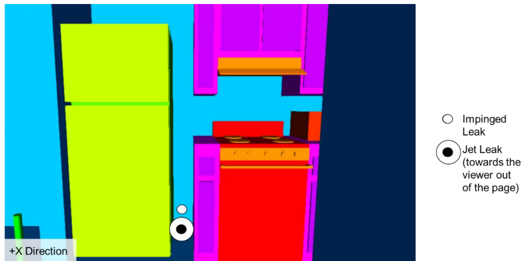
Figure 2.6: Range leak location.
