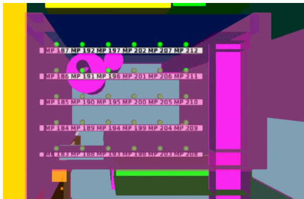
Figure A.23: Detectors on the ceiling in the utility room.
